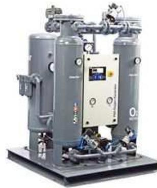
Oxygen Gas Plant work with PSA (Pressure Swing Adsorption) technology. Using this technology, we produce oxygen gas plants that are highly economical and require low maintenance and produce the desired results in a hassle-free manner. These generators absorb nitrogen with the help of two absorption vessels that are filled with most efficient X type zeolite molecular sieves responsible for nitrogen absorption.
